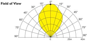
To meet the requirements of EN54:10 clause 5.4, where the ratio of the response points Dmax:Dmin should not exceed 1.41, the horizontal and vertical viewing angles  $\alpha$ max should not exceed  $\pm 30^{\circ}$ .
